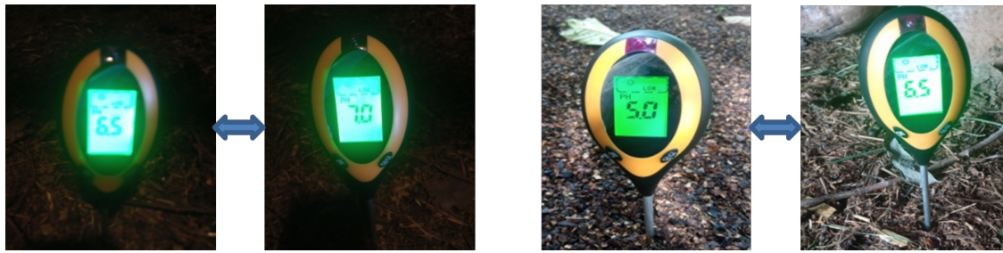
Figure 2. Use of pH Meter in Measuring Compost pH
