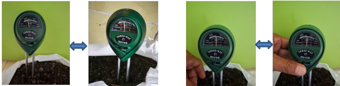
Figure 3. Measuring Compost Moisture Content Using a Three-Way Meter
